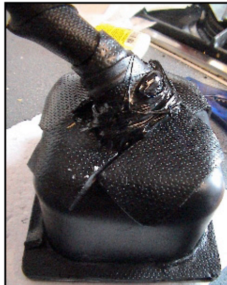
Audio Acoustics adhere's special material to the driver assemblies to control mechanical resonances. The photo above shows the tweeter...
